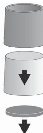
\* For easy processing, the BEGO combi duplicating flask (order no. 52090) can be used. Due to the special form of this flask, a model with fitting base plate will be produced during duplicating with gel. Thus, the hard rubber plate of the mould former is no longer necessary.
